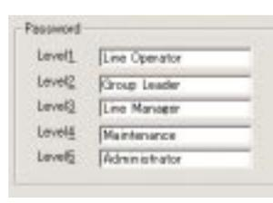
Operator passwords are managed in 5 levels. Passwords can be up to 16 characters long and the access rights increase as the level number increases.
