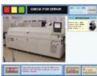
When an error occurs, the location of the error can be shown realistically in a picture.
