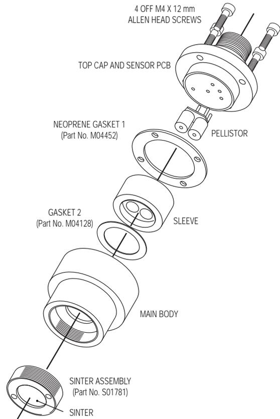
Diagram 2: 96HD sensor housing with flammable sensor
