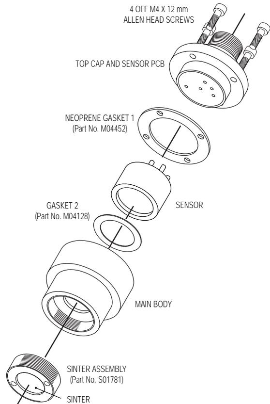
Diagram 3: 96HD sensor housing with toxic sensor
