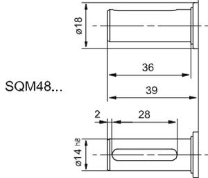
Groove for parallel key A5x3x28 to DIN 6885 T3
