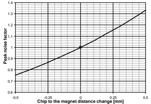
Fig. 14: Peak noise factor Vs Distance change
