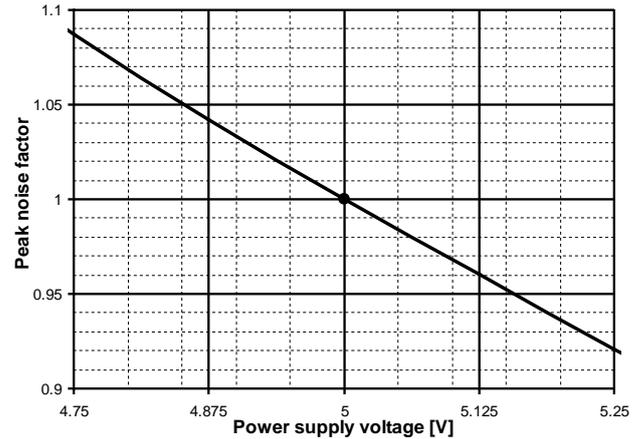
Fig. 12: Peak noise factor Vs Power supply
