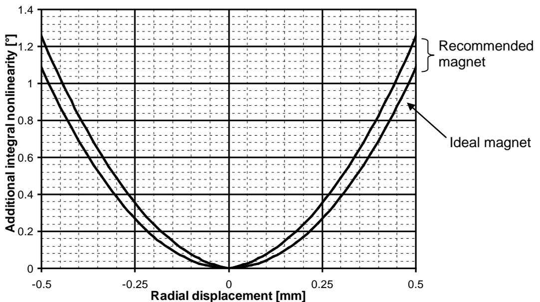
Fig. 21: Additional integral nonlinearity error caused by magnet displacement
