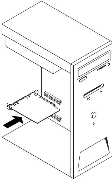
6. Screw the mounting bracket of the GPIB board to the back panel rail of the computer.
