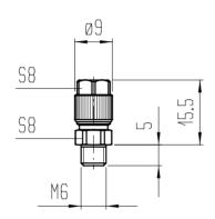
Werkstoff: Ms58, gal. vernickelt
