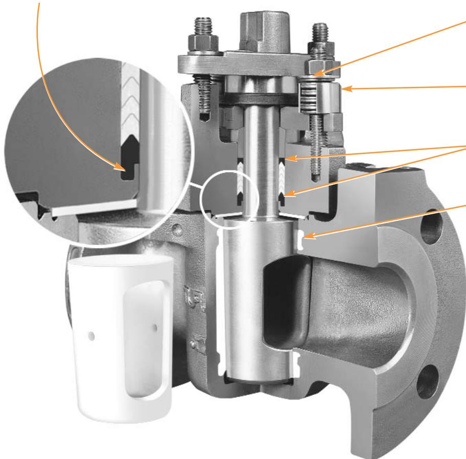
Live loaded spring washers provide a constant, uniform pressure on the packing. This is especially important during thermal cycling.
