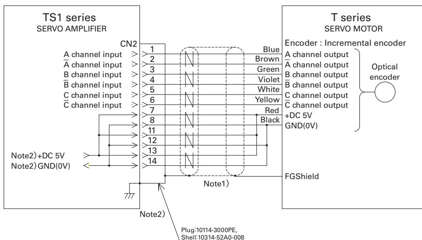
Note 1) For the parts marked
