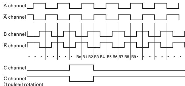
Output cross-phase difference:  $R_n$  ( $n=1$  to pulse number  $\times 4$ )
