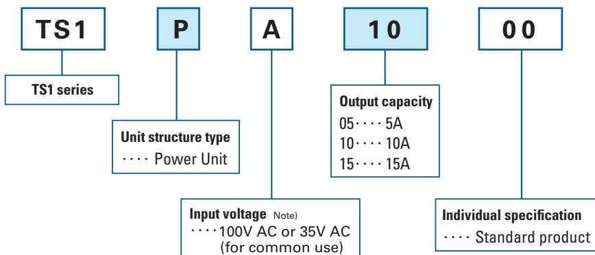
Note) Supply AC100V if the motor winding specification is 75V series and supply AC35V if it is 24V series.
