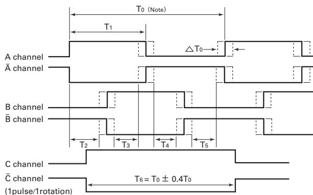
Notice) "T<sub>0</sub>" is the average value of each cycle during one encoder rotation at a constant speed.
