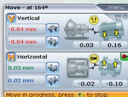
ROTALIGN® smart RS5 EX is a high-end laser shaft alignment system designed for the use in hazardous areas. It is ATEX/IECEx certified for zone 1.
