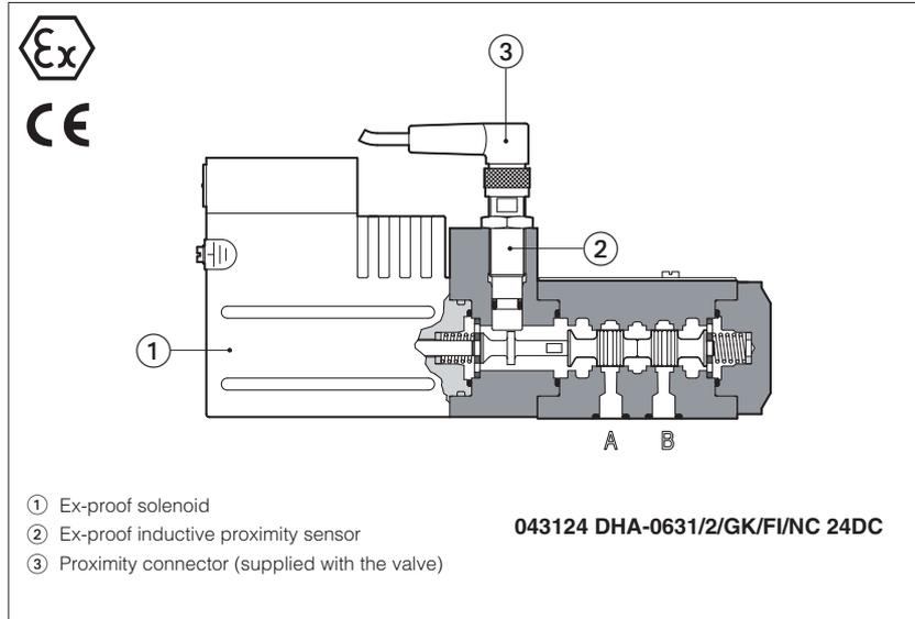
Ex-proof on/off solenoid valves equipped with proximity sensor for the spool position monitoring, certified according to ATEX 94/9/EC, protection mode: Ex II 2 GD Ex d IIC T6/T4/T3 category 2, zone 1, and 2 (see section 4).
