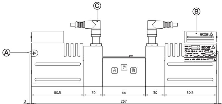
(A) = screw terminal for additional equipotential grounding
