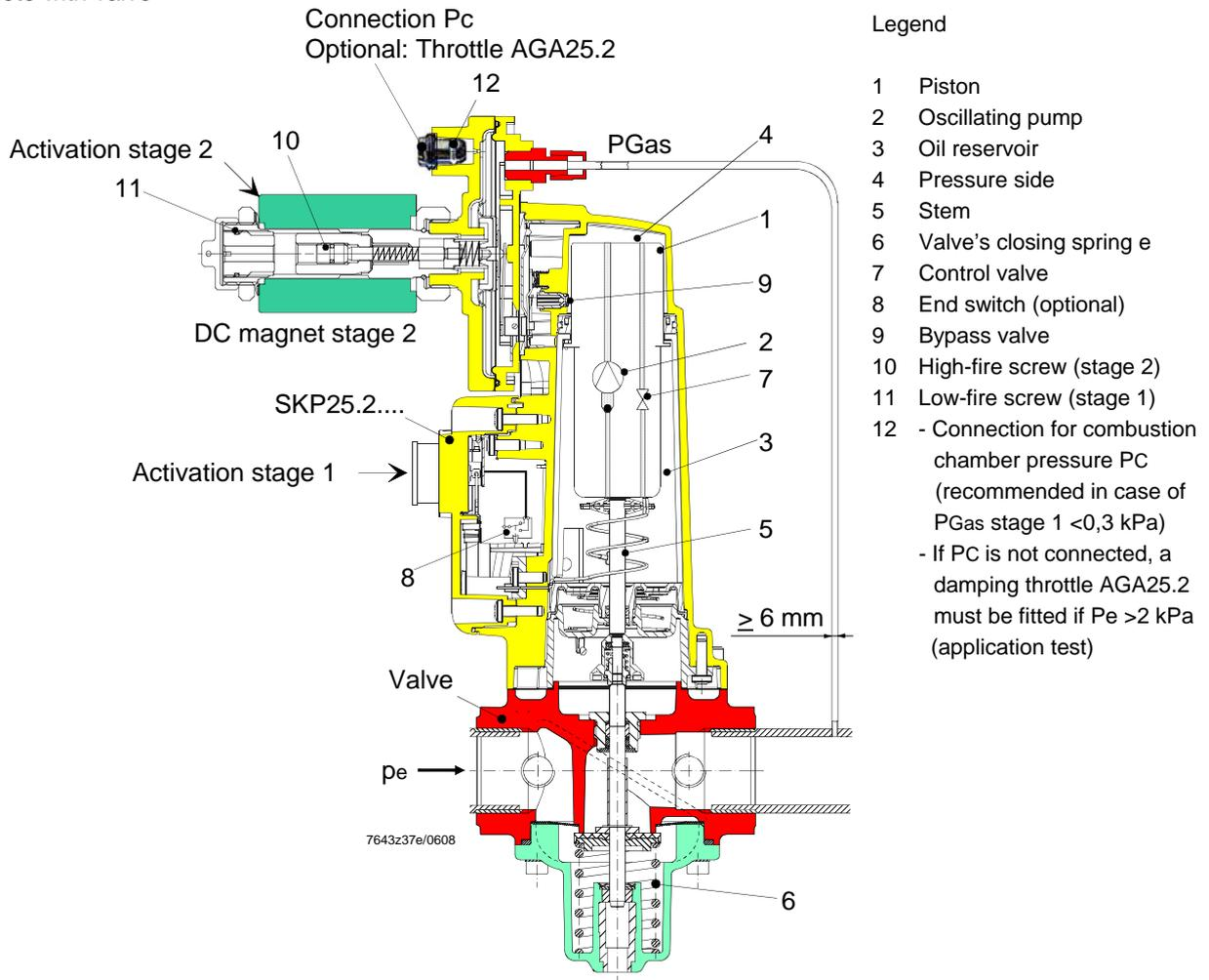
Setpoint adjustment «P<sub>Gas</sub>» is made manually by turning the setting screws (10 and 11), which act on the setpoint spring.
