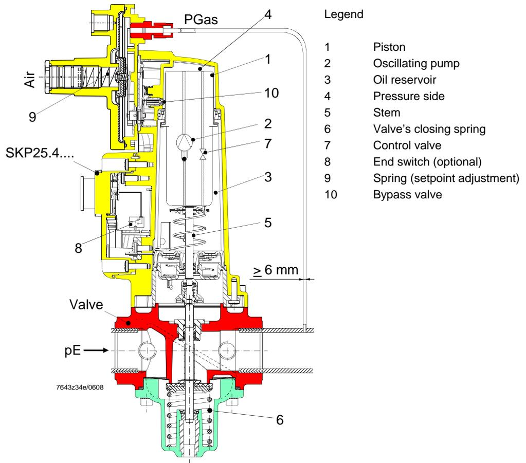
Setpoint adjustment «PGas» is made manually by turning the setting screw, which acts on the setpoint spring (for setpoint springs, also refer to «Accessories»).
