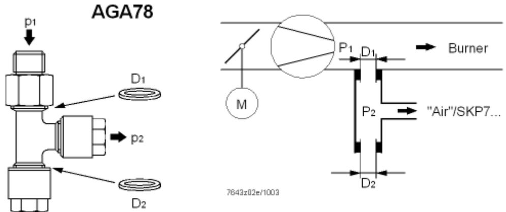
The reducing T-piece AGA78 is supplied ready for mounting, with  $D_1 = 1.5 \text{ mm}$  and  $D_2 = 1.7 \text{ mm}$ .
