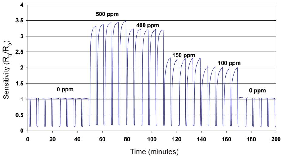
Real-time sensitivity data over range 100 - 500ppm CO in 50% rh air. Sensor operating in 2-temperature mode, pulsing between 5 mins at 400°C for 5 mins and 525°C for 1 min.
