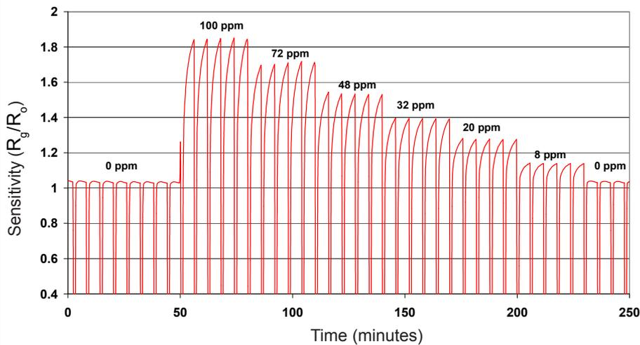
Real-time sensitivity data for 8 - 100ppm CO in 50% rh air. Sensor operating in 2-temperature mode, pulsing between 400°C for 5 min and 525°C for 1 min.
