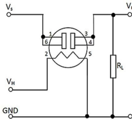
Pins on the measuring circuit, shown in Figure 8, correspond with the pin numbers in Figure 1, 2 & 3 above.
