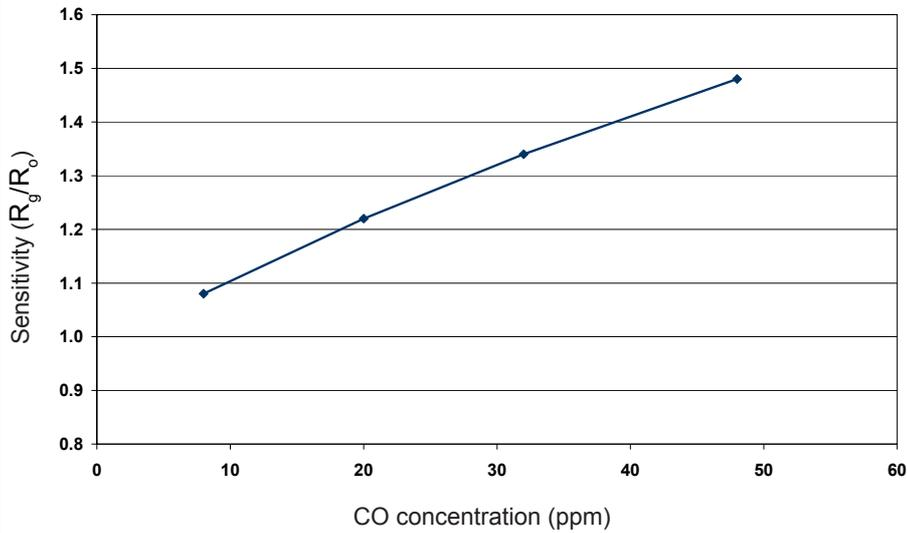
Sensitivity over range 8-50ppm CO operating in 2-temperature mode with a 5:1 cycle ratio of sensing (400°C) and resetting (525°C). Linear behaviour is observed.
