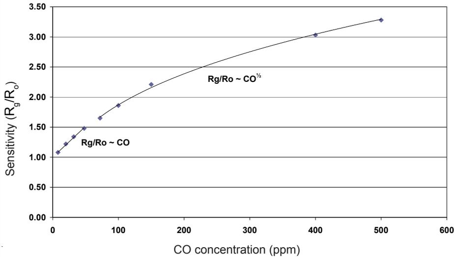
Sensitivity over range 8 - 500ppm CO operating in 2-temperature mode with a 5:1 cycle ratio of sensing (400°C) and resetting (525°C). Note linear behaviour <50ppm and power law behaviour >50ppm.
