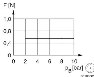
F = actuating force at the rear end of the spring-loaded rod
