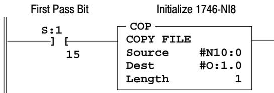
On power up, the first pass bit (S:1/15) is set for one scan, enabling the COPY instruction that transfers the channel configuration word 0. This configures and enables the channel.
