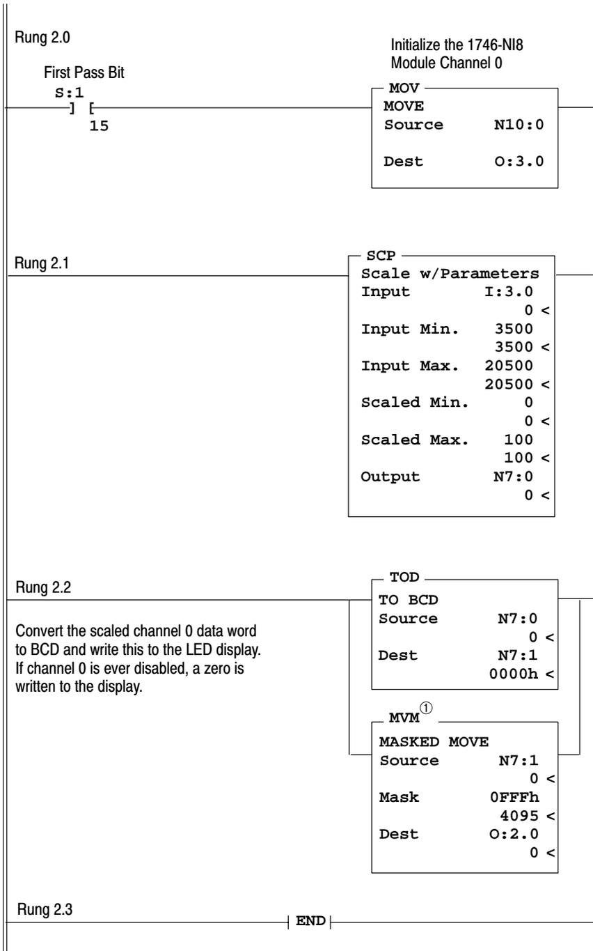
① The use of the masked move instruction with the 0FFF mask allows you to use outputs 12, 13, 14, and 15 for other output devices in your system. The 7-segment display uses outputs 0-11.
