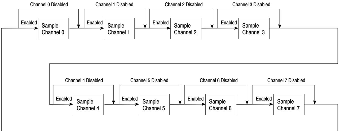
The following table shows the module update time. The module update time is the same regardless of the filter frequency. The fastest module update time occurs when only one channel is enabled. The slowest module update time occurs when 8 channels are enabled.
