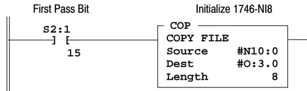
On power up, bit S2:1/15 is set for the first program scan, and integer file N10 is sent to the eight 1746-NI8 channel configuration words.
