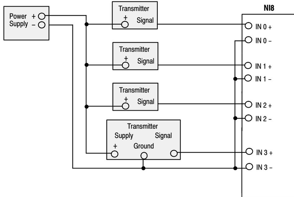
**Wiring Schematics for 2, 3, and 4-Wire Analog Input Devices**
