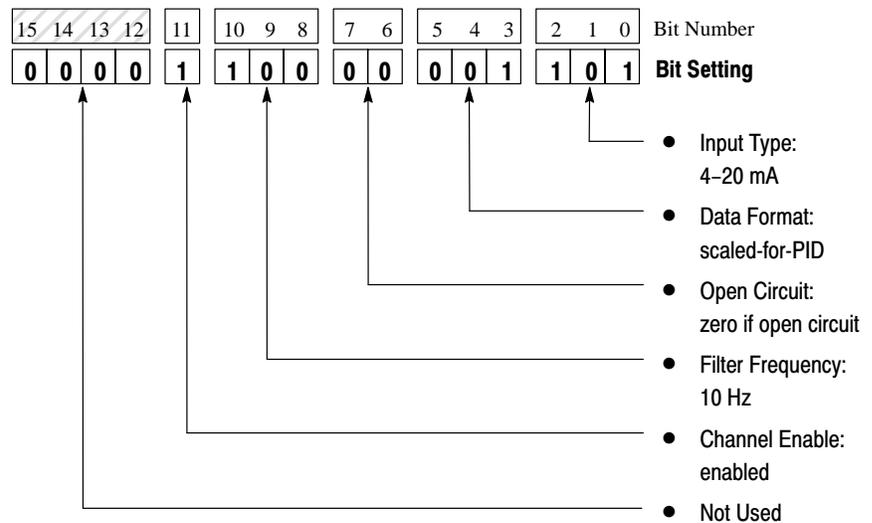
This example transfers configuration data and sets the channel enable bits of all eight channels with a single File Copy instruction.
