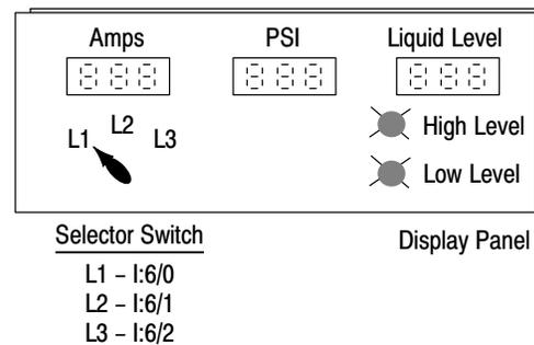
3. If the liquid level goes below the low level set point, turn on the low level warning light, and if the liquid level goes above the high level set point, turn on the high level warning light.
