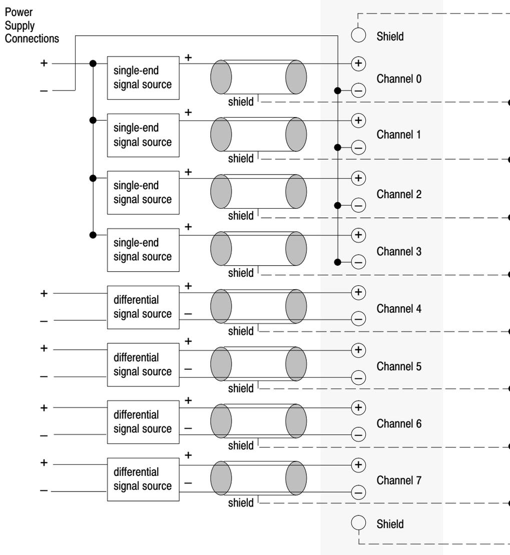
**Wiring Schematic for Single-ended Analog Input Connections**
