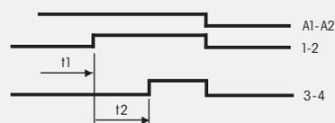
When the control voltage is applied, the time lapse  $T_1$  starts between 0 and 60 seconds. At the end of the time lapse, contact 1-2 closes and time lapse  $T_2$  starts between 0 and 60 seconds. At the end of this time lapse, contact 3-4 closes. After an interval, the time lapse starts again at  $T_1$ .
