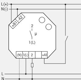
If N is connected, the zero passage switching is active.
