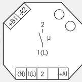
**1 NO contact potential free 10 A/250 V AC. Incandescent lamps 2000 W\*. Standby loss 0.02 – 0.4 watt only.**
