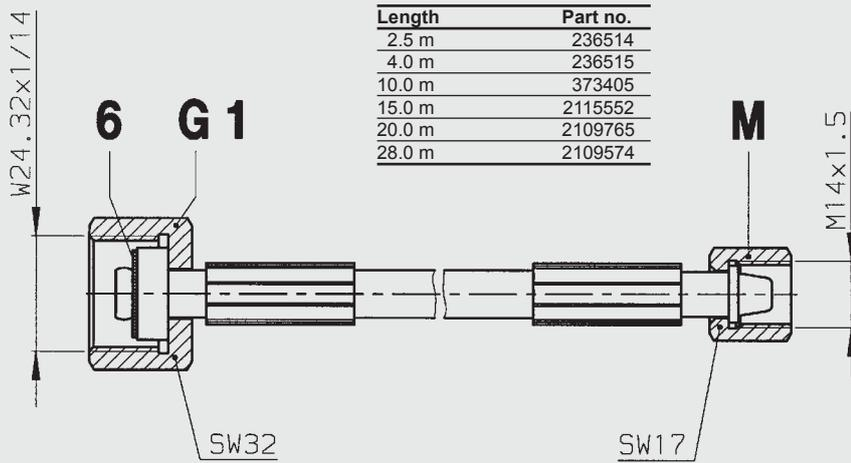
Charging hoses are suitable for the particular maximum permitted operating pressure marked on them and 10,000 charging processes. (HYDAC charging hoses comply with the EC Machinery Directive and with DIN EN 982 and DIN EN 853 to 857)
