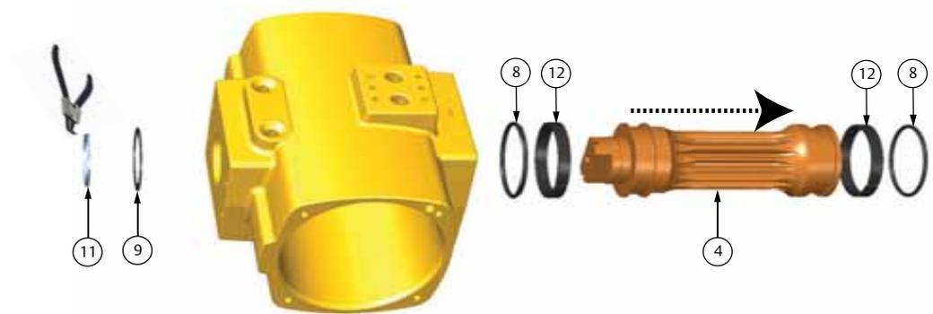
Table 12. Recommended circlip pliers according DIN 5254 (or equal) for shaft circlips.
