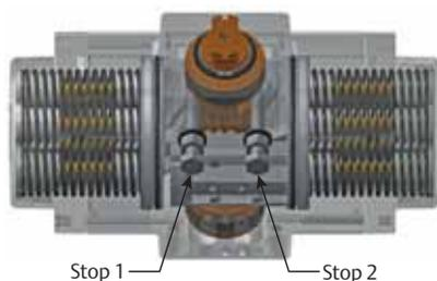
3. Turn the "closed" stop clockwise to reduce or counterclockwise to increase the travel. Consult chapter 5.1.3 (angular displacement of the pinion), to define how far the limit stop must be turned in or out.
