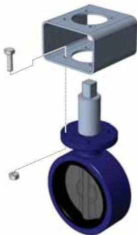
5. Install the actuator to the bracket. Tighten all bolts and apply the correct torque (refer to Table 8).
