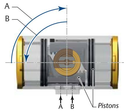
A = Rotation when central air chamber is pressurized.
