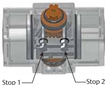
4. Turn the "closed" stop clockwise to reduce or counterclockwise to increase the travel. Consult chapter 5.1.3 (angular displacement of the pinion), to define how far the limit stop must be turned in or out.
