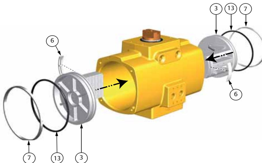
3. Align the pinion (see Figure 26) so that the teeth on the pinion will pick up the pistons rack teeth when turning the pinion. Note the position of the pinion top slot and the cam on the pinion top:
