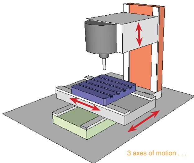
... and multiple potential positioning errors on each axis (and between axes)
