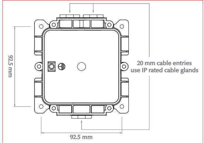
Figure 2 XP95® Intrinsically Safe Manual Call Point dimensional drawing
