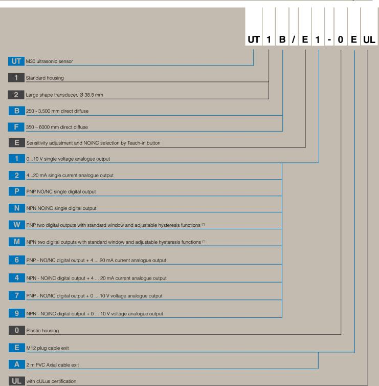
$<sup>\</sup>ensuremath{^{(\mbox{\tiny '})}}$  The two functions switching is possible pressing the Teach-in button.
