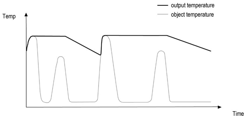
**Figure 32: Linear Signal Drop (decay mode)**
