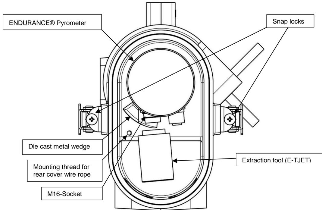
**Figure 80: Extraction tool (E-TJET) attached to Endurance® M16 Connector**
