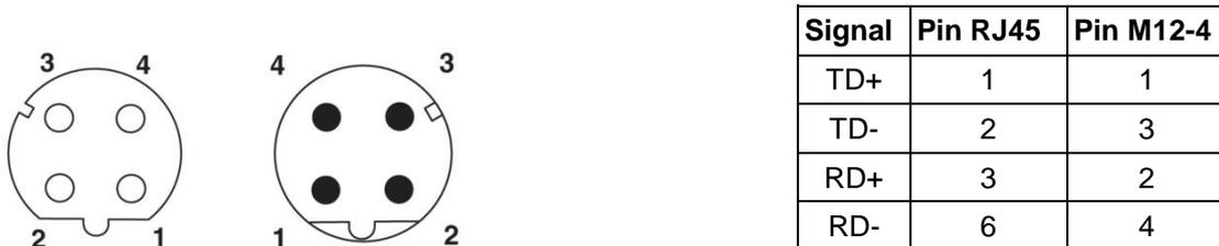
Figure 11: M12 Socket (left) and the corresponding cable plug (right)
