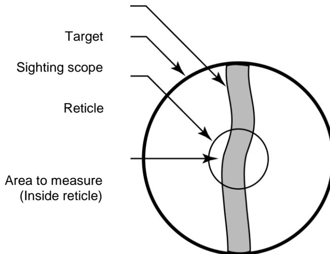
**Figure 8: Sensor Eyepiece and Reticle**
