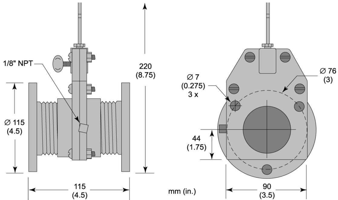
**Figure 72: Dimensions of the Blast Gate Assembly**
