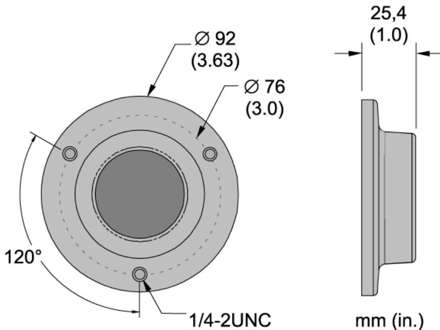
**Figure 75: Mounting Flange for Sighting Tube (E-MST)**
