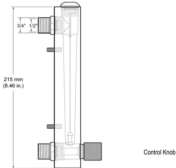
**Figure 83: Dimensions of Cooling Air Flow Regulator (E-CAFR-7)**
