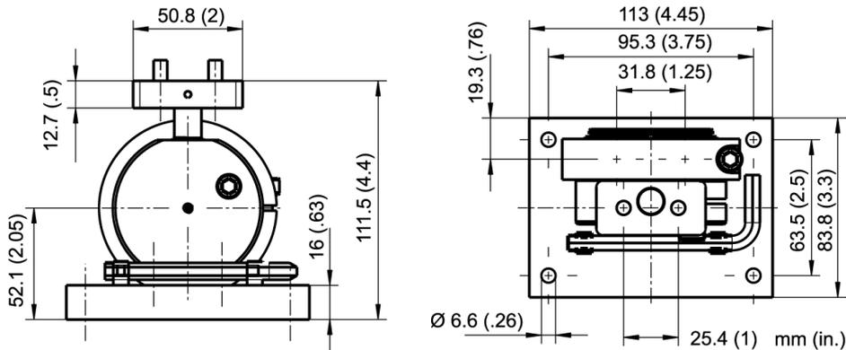
**Figure 70: Adjustable Mounting Base for ThermoJacket (E-MB)**
