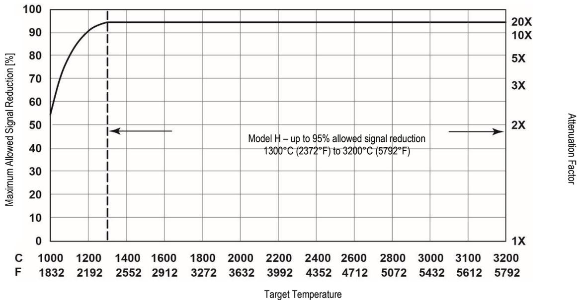
**Figure 85: Model H Percentage of Allowed Signal Reduction**
