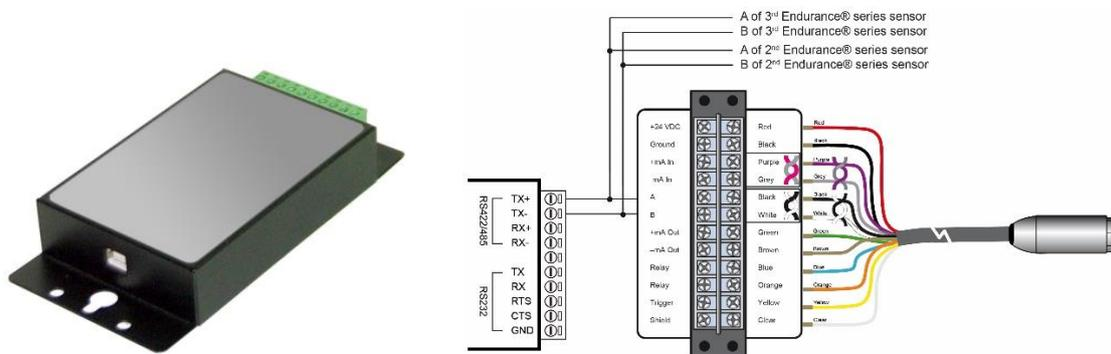
**Figure 16: USB/RS485 Converter**
