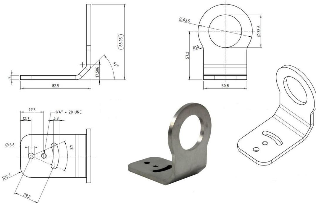
**Figure 56: Drawing and Photo of Fixed Bracket (E-FB)**
