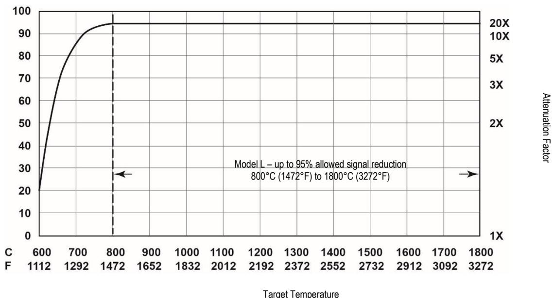
Figure 84: Model L Percentage of Allowed Signal Reduction
