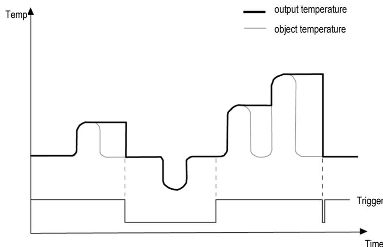
**Figure 30: Peak Hold reset by external Trigger signal**
