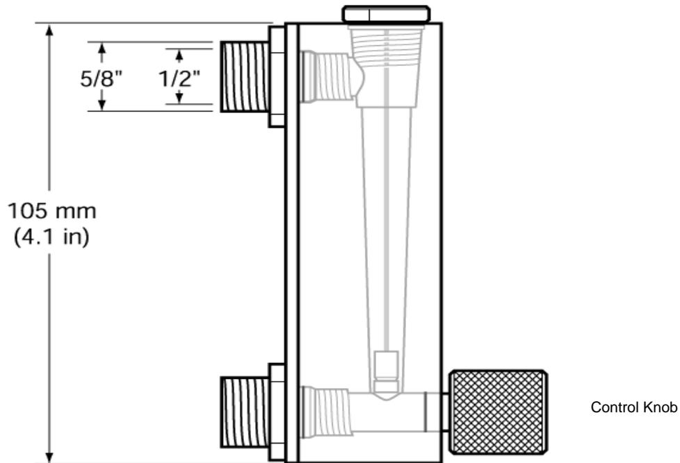
**Figure 81: Water Flow Regulator (E-WR)**
