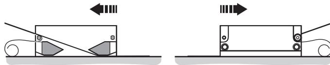
3. Ensure that the end of the scale is in line with the 'START' position on the axis and slowly and smoothly take the applicator through its full axial run, ensuring that the backing paper is pulled manually from the scale.
