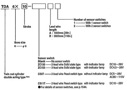
Note: In the standard cylinder, a magnet for sensor switch is built-in.
