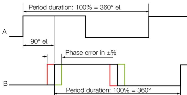
El. phase offset: 90° ± max. phase error 7,5% of a pulse length
