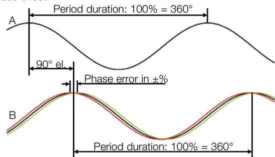
El. phase offset: 90° ± max. phase error 7,5% of a pulse length
