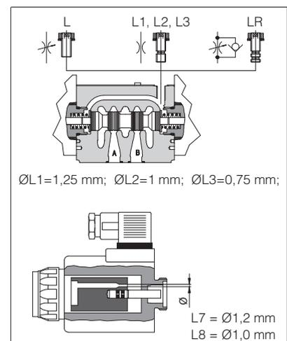
**11 COILS TYPE CAE WITH SPECIAL CONNECTORS** (only for 12DC, 14DC, 24DC and 28DC)
