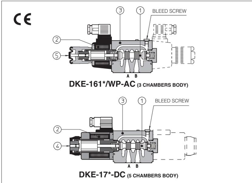
Spool type, two or three position direct operated valves with threaded solenoids certified according to the North American standard **cURus**.
