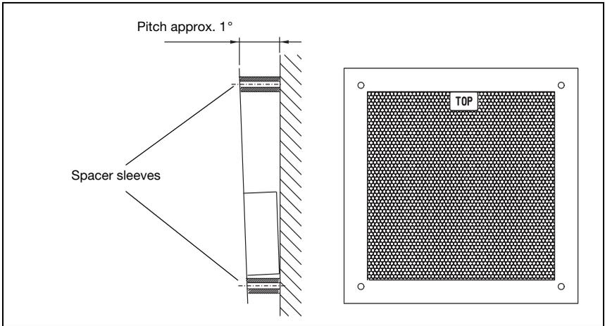
Figure 1.6: Pitch of the heated reflector
