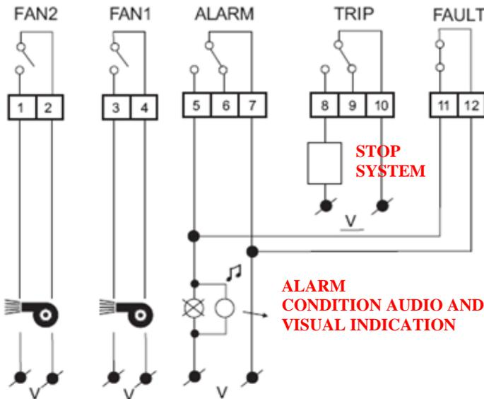
Output relay with 10A-250Vac-res COS $\Phi$ =1 contacts.
