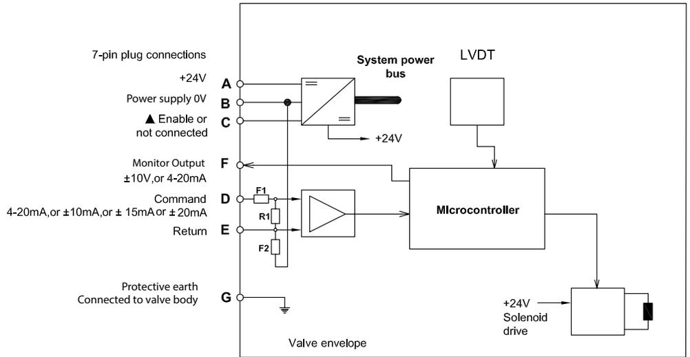
▲ Pin C is used for a valve enable signal with electrical connections Field = H or R
