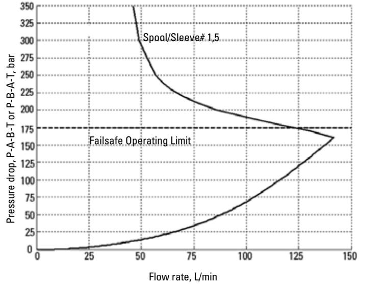
**Operating Limit:** When operating the valve beyond the operating pressure limit, spool may not return to failsafe when power is removed
