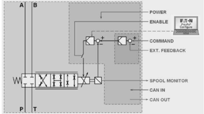
Distributed motion control, taking advantage of the available axis-control function embedded in the valve controller for AxisPro level 2 and 3. Command can be analog via the 7-pin connector or via CANopen using the M12 connections illustrated on page 12.
