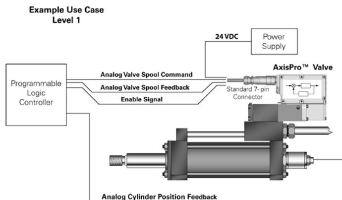
AxisPro level 1 valves, such as KBS1-05 (ISO size 5), can be used to control machine motions in open loop or closed loop control applications. The valve receives its analog command input on the 7-pin, main, connector from an external axis control device.
