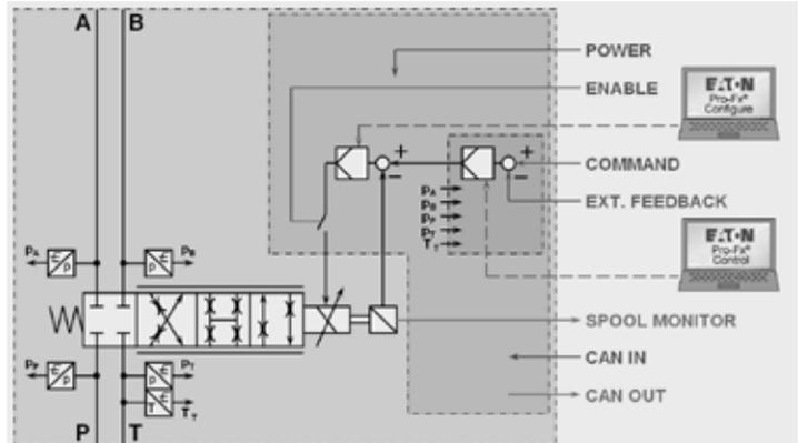
Selecting the CW-option allows user specific applications to be developed in Eaton's Pro-FX Control software tool, which is based on the popular CODESYS development environment.
