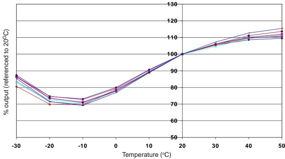
Figure 2 shows the temperature dependence of sensitivity at 2ppm NO<sub>2</sub>.
