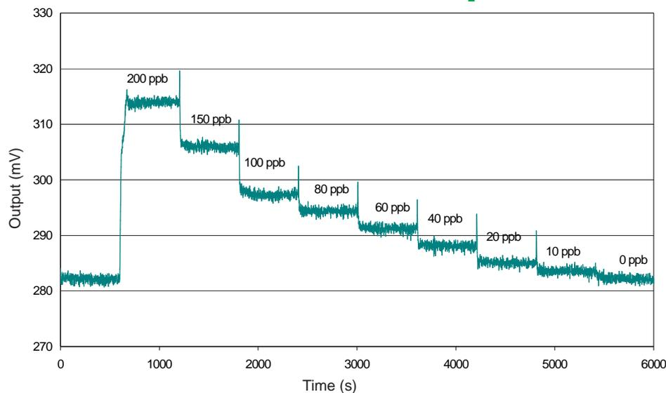
Figure 4 shows response from from 200ppb NO<sub>2</sub> to 0ppb NO<sub>2</sub>.
