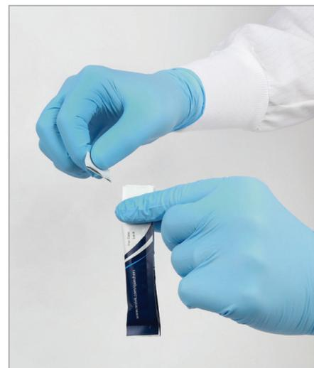
**6.** Open the extraction salt packet by tearing straight across the pre-cut slit.
