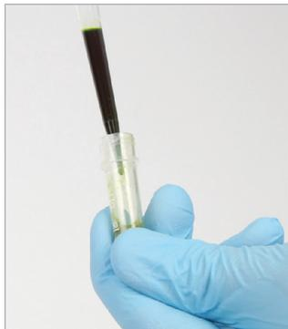
**1.** Open the cap of a dSPE tube and transfer in an aliquot of the supernatant (organic solvent layer) of the centrifuged extracts from Stage 1 (see table for transfer volume).
