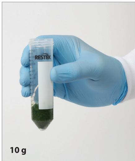
**2.** Open the cap of a 50 mL centrifuge tube and weigh in 10 g of homogenized sample. Note that the 10 g sample size is for matrices >80% water. For drier materials, consult the method or other resources.
