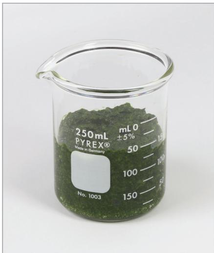
**1.** Homogenize the food matrix to generate a uniform sample that is representative of the product. For commodities with more than 5% fat (w/w), see the specialized sample preparation procedure in the source method [2, 3].
