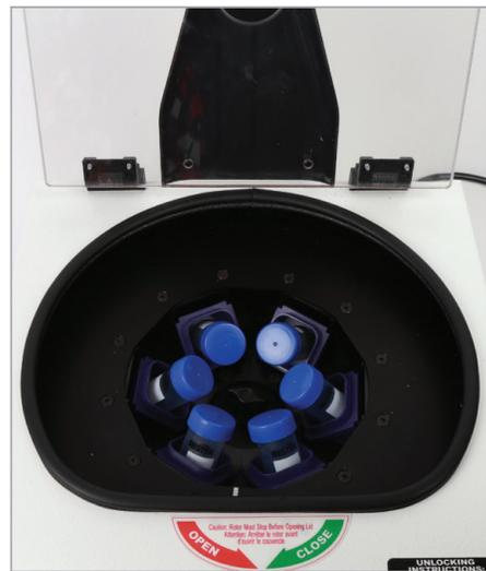
**9.** Centrifuge the 50 mL tube per reference [2] or [3] to separate the layers.
