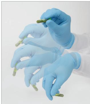
**2.** Immediately recap the dSPE tube and vortex or shake it vigorously by hand (see table for shake time).
