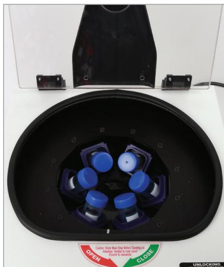
**8.** Centrifuge the 50 mL tube per reference [4] to separate the layers.
