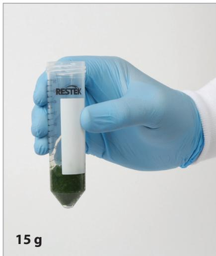
**2.** Open the cap of a 50 mL centrifuge tube and weigh in 15 g of homogenized sample. Note that the 15 g sample size is for matrices >80% water. For drier materials, consult the method or other resources.
