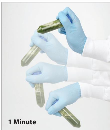
**7.** Immediately recap the 50 mL tube and vortex or shake it vigorously by hand for 1 minute.
