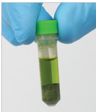
**4.** After centrifugation is complete, transfer the supernatant from the dSPE tube to an autosampler vial, make any final adjustments if required, and test using an appropriate GC or LC method.
