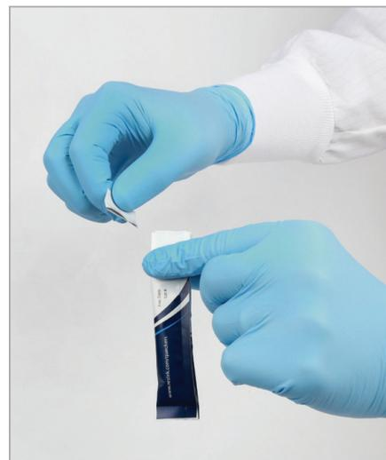
**5.** Open the extraction salt packet by tearing straight across the precut slit.
