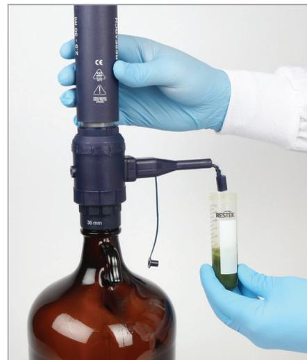
**3.** Add 15 mL of a 1% acetic acid solution in acetonitrile (v/v).
