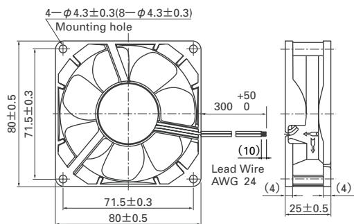
**Reference dimension of mounting holes and vent opening (unit : mm)**
