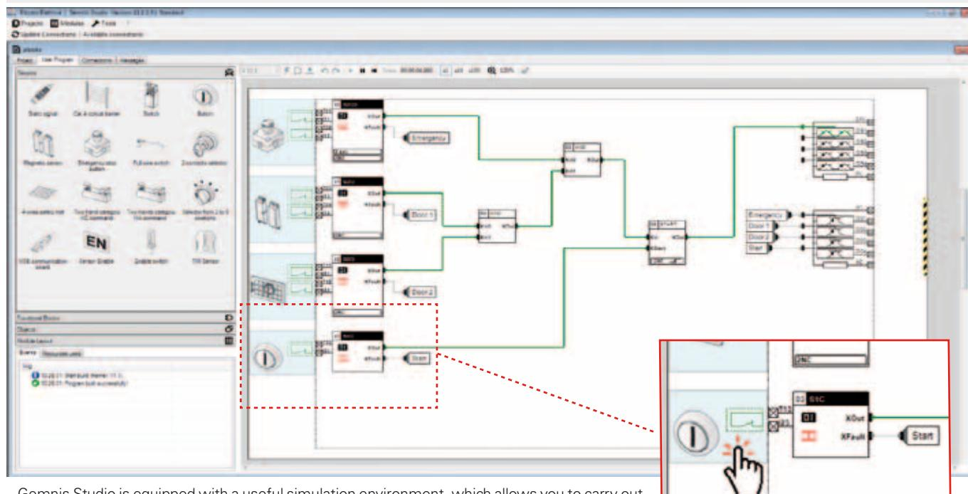
Gemnis Studio is equipped with a useful simulation environment, which allows you to carry out tests on your application program under development and check its correct operation before you install it to a module. To run an application program simulation during the development phase, simply press the Start button on the toolbar at the top of the desktop. If the application program cannot compile, the simulation will not run.
