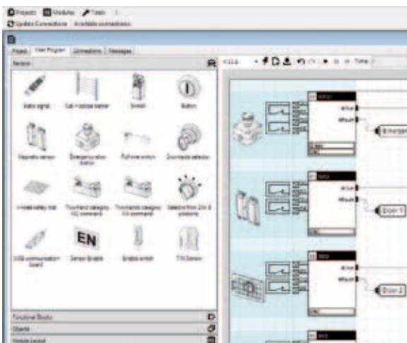
The sensor zone indicates the external device types which can be connected to the module terminals, and all the parameters needed to define them.
