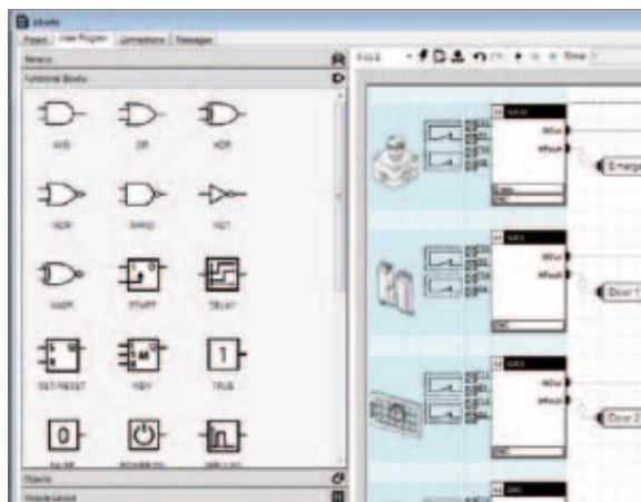
The function blocks represent all the logic functions required to process the data flow between sensors and outputs.
