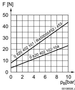
$F$  = actuating force $P_B$  = Working pressure**Dimensions, Fig. 1, Basic valve**
