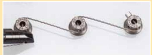
Correct tension is applied with the tool.
