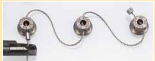
The ferrule is threaded on the cable and the cable is inserted through the tool nose.
