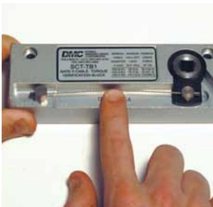
Safe-T-Cable® should remain in place during application of the measured force. If the ferrule pops off the cable, the crimp is unacceptable and the tool indenter should be adjusted. If the ferrule remains attached to the cable, recheck the cable tension as before. If the cable now touches either the side or the bottom surface of the Torque Verification Block, the crimp is unacceptable and the tool indenter should be adjusted.
