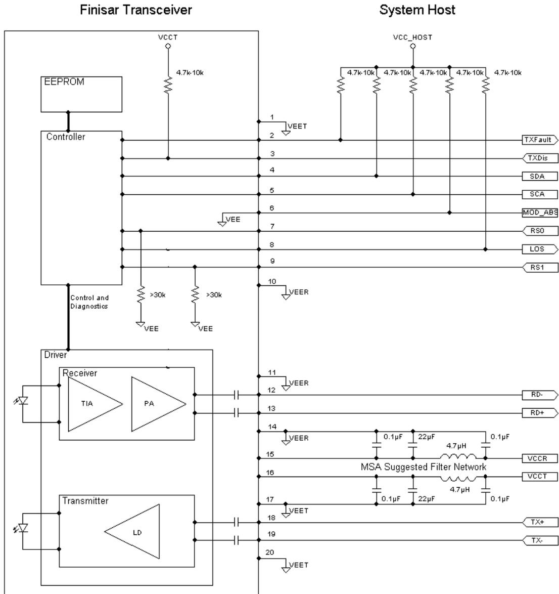
**Figure 6-Host-Module Interface**
