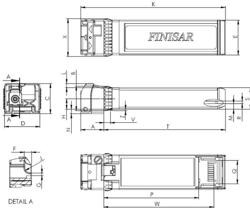
**Figure 2. FTLX2672D327/FTLX2672D333 Mechanical Dimensions**
