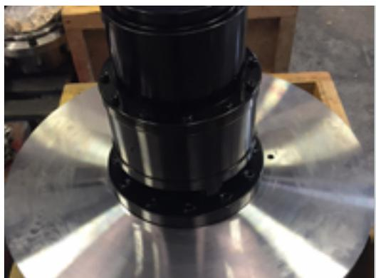
Gear coupling with brake disc.
