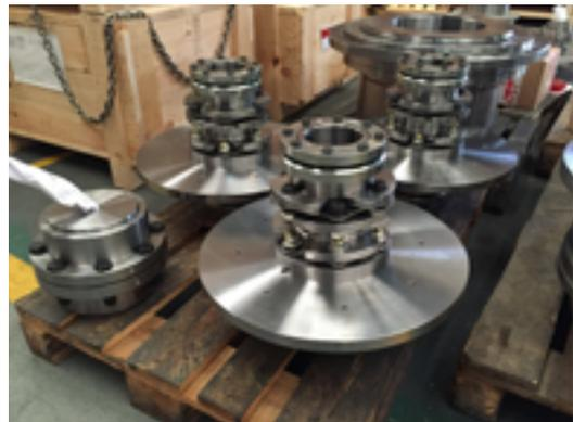
Disc pack configuration with brake disc.
