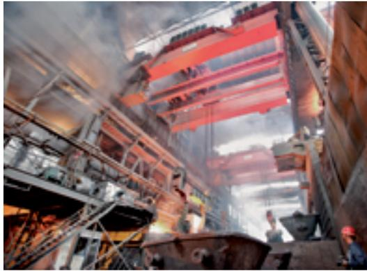
Travelling crane in steel plant.
