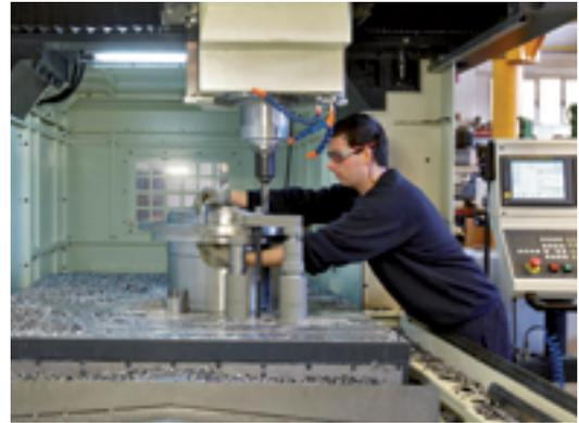
Machining of barrel coupling's hub.
