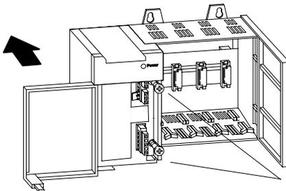
Use these screws to fasten the power supply to the chassis with 1.2 Nm (11 lb-in) torque, max.
