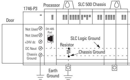
5. **(Optional)** For the 1746-P1, 1746-P2, 1746-P4, 1746-P5, and 1746-P6 power supplies, use PWR OUT +24V dc and PWR OUT COM terminals to power 24V dc sensors and loads. The terminals on the 1746-P1, 1746-P2, 1746-P5, and 1746-P6 power supplies provide an isolated, non-fused 200 mA, 24V dc power supply. The terminals on the 1746-P4 power supply provide an isolated, non-fused 1A, 24V dc power supply. (The 1746-P3 and 1746-P7 power supplies do not provide for an external power source.)
