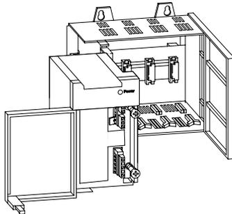
2. Slide the power supply in until it is flush with the chassis. Then fasten the power supply to the chassis.
