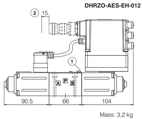
① = Screw for air bleeding: at the first valve commissioning the air eventually trapped inside the solenoid must be bled-off through the screw ①
