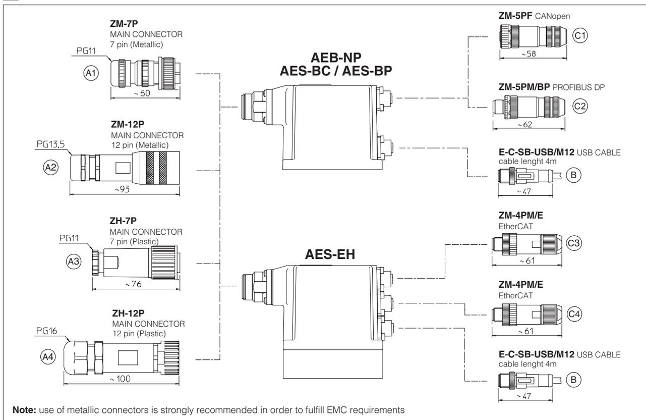
12 MODEL CODES OF MAIN CONNECTORS AND COMMUNICATION CONNECTORS - to be ordered separately
