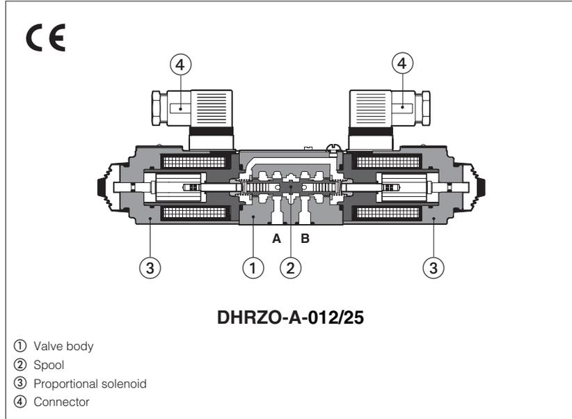
DHRZO are 3 way, proportional pressure reducing valves, direct operated, with standard ISO 4401 size 06 mounting surface
