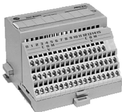
Each FLEX I/O™ module requires a terminal base unit that snaps onto the DIN rail to the right of the I/O adapter. The terminal bases provide terminal connection points for I/O wiring and plug together to form the backplane. They are available with cage, screw or spring - clamp terminations.
