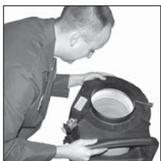
Inspect the engine air cleaner.
