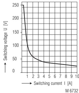
Limit curve for arc-free operation with resistive load
