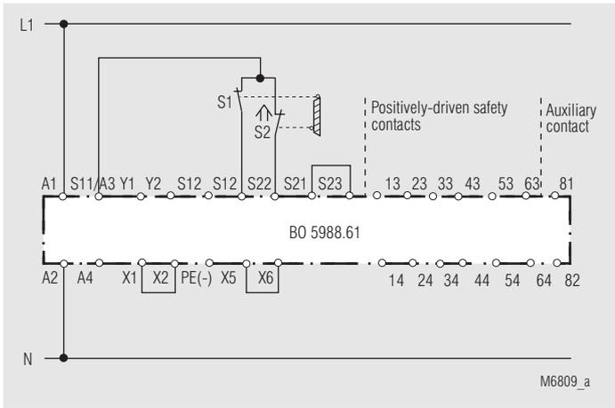
Two-channel monitoring of a safety gate. S1 must not close before S2
