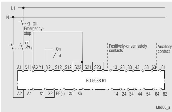
Two-pole emergency stop circuit with emergency stop control device in the supply circuit. Application for long emergency stop loops where the control voltage drops below the minimum voltage of 21 V.
