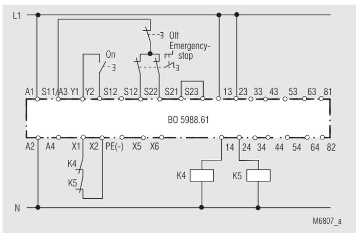
Contact reinforcement by external contactors, two-channel. The output contacts can be reinforced by external contactors with positively-driven contacts for switching currents > 8 A. Functioning of the external contactors is monitored by looping the NC contacts into the closing circuit (terminals X1 - X2).
