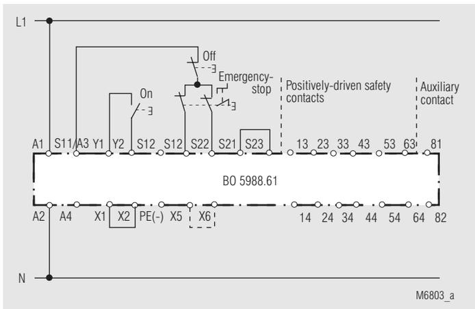
Two-channel emergency stop circuit without cross fault detection. Activation via On pushbutton. - - - Jumper X5 - X6: A jumper must be fitted X5 - X6 for the automatic On function. The On pushbutton is not required.
