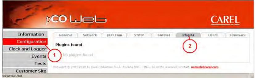
Figure 9.m - Installing / uninstalling the Plugins
