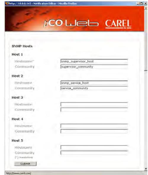
Figure 4.o – SNMP Hosts configuration for sending the TRAP messages
