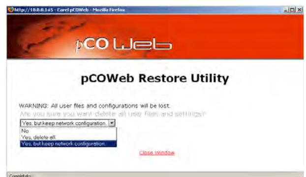
Figure 9.i – Restoring *pCOWeb* to the default situation
