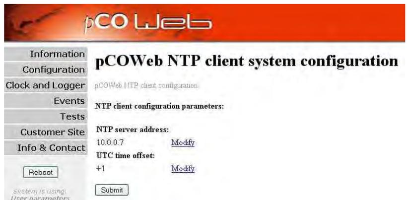
Figure 9.s – Page for setting the “NTP” Plugin parameters
