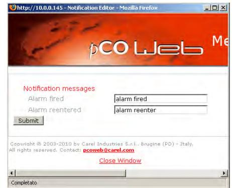
Figure 4.r – Setting the strings sent for Activation - Return
