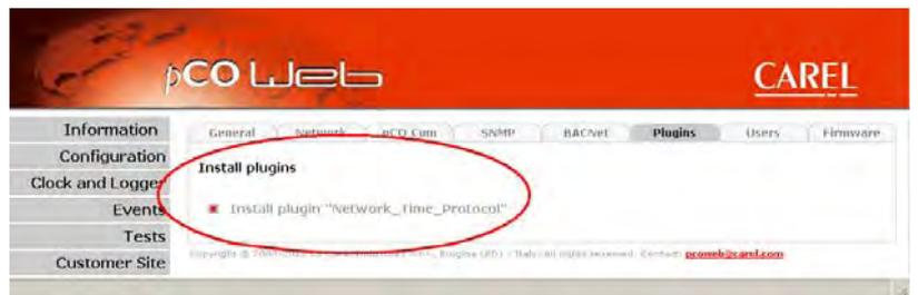
Figure 9.o – Install/Uninstall Plugin page: list of Plugins ready to be installed
