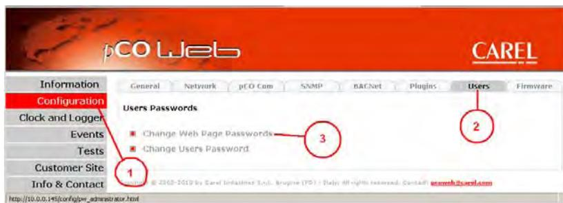
Figure 9.v – Protection and access control
