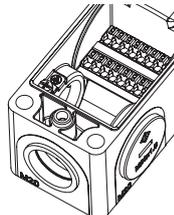
The switch is provided with a PUSH-IN type spring connection system on the inside. This technology allows quick handy wiring, since the wire simply needs to be inserted in the appropriate hole for it to be secured and for the electrical connection to be established. Such operation can be carried out without the help of any tool but just using rigid or flexible wires with a tip. The wires can be released by pressing the appropriate wire-releasing push-buttons.
