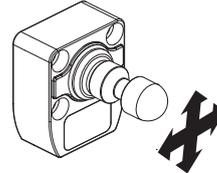
All the NG series actuators are articulated, and allow the pin to match the centring hole found in the switch. This way there is no need for precise actuator-switch aligning operations during the fitting stage. Moreover, thanks to its flexibility, this device can be used on doors with an activating range up to 150 mm, without having to tilt the pin beforehand.
