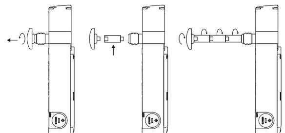
Metal extensions can be combined together until the required length is obtained. Do not exceed an overall length of 500 mm between the release button and the switch.
