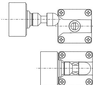
The switch is provided with a wide centring inlet for the actuator pin. Such solution makes it easier to align the actuator with the hole found in the head during the fitting stage. Moreover, this solution drastically reduces any probable collisions between the actuator and the switch, also allowing it to be fitted on inaccurate doors.
