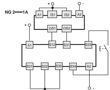
Wiring with safety modules CS MF●●●●●, CS MP●●●●●
