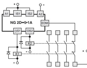
The NG 2D••5•1A version maintains the safety and operating characteristics of the NG series, and allows the control of **the NC contacts of contactors or of forcedly guided relays**, which are controlled by the safety outputs of the switches.
