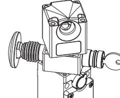
The head and the release device can be adjusted but cannot be detached from each other. This makes the switch more secure since the installer need not worry about how to assemble the various pieces, and the switch is less likely to become damaged (small parts being lost, dirt getting in etc.).
