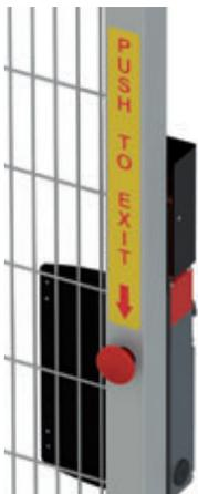
Polycarbonate yellow adhesive, rectangular 300x32 mm, red writing. Applied on the jamb internal part it helps finding the emergency release push button.
