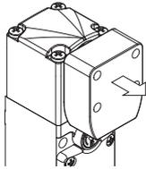
The inside of each switch features a device which holds the actuator in its closed position. Ideal for all those applications where several doors are unlocked simultaneously, but only one is actually opened. The device keeps all the unlocked doors in their position, stopping any vibrations or gusts of wind from opening them.
