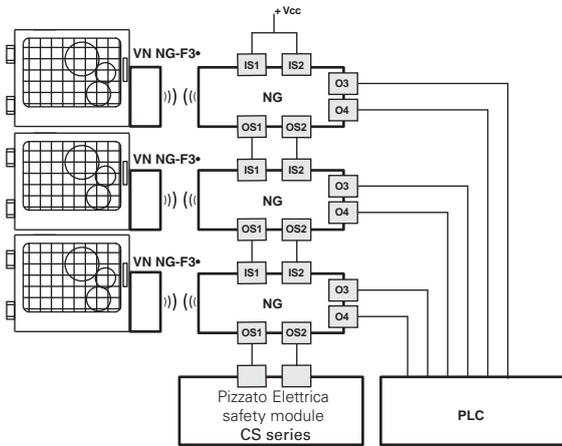
Possible connection in series of several switches in order to simplify the safety system wiring, prior evaluation of the outputs of the last switch in the chain by means of a Pizzato Elettrica safety module (see table for safety modules to be combined). Each NG series switch is provided with two signalling outputs which are activated when the guard is closed (O3) or locked (O4). This piece of information can be managed by a PLC, depending on the specific requirements of the system installed.
