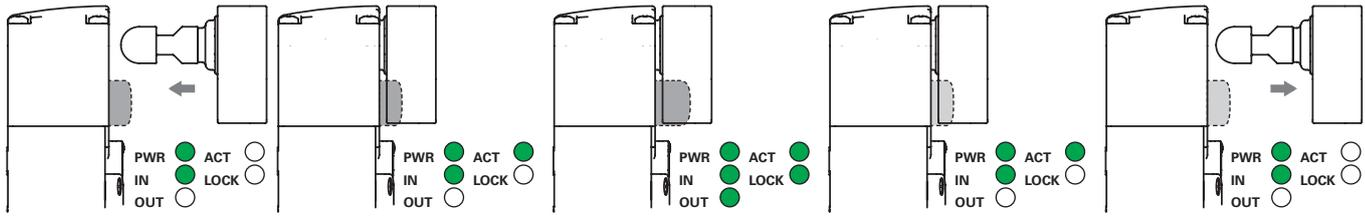
The switch is supplied with power (PWR LED on, green), the IS1 and IS2 inputs are enabled (IN LED on, green), the OS1 and OS2 safety outputs are disabled (OUT LED off). The actuator is outside the activation area (ACT LED off).
