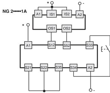
Wiring with safety modules CS AR-05●●●● / CS AR-06●●●●
