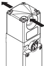
The switch is provided with a through hole for inserting the actuator and, thanks to this peculiarity, any dust which may go inside the actuator hole can always come out of the opposite side instead of being left there. Moreover, the lock pin is provided with an external diaphragm gasket which makes it suitable for any environment where dust is present.
