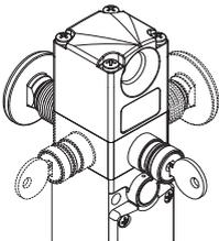
The lock release device allows the actuator release only to staff who possess the actuating key. It also works in absence of power supply and once actuated it prevents the guard arrest.
