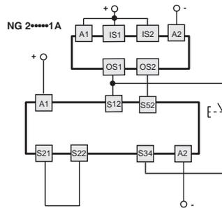
Wiring with safety modules CS AT-0●●●●● / CS AT-1●●●●●
