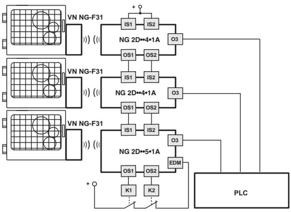
This model, having safety inputs IS, can be connected at the end of a series of NG switches, maximum 32 devices, while maintaining the maximum safety levels PL e in conformity with EN ISO 13849-1 and SIL 3 according to EN 62061. This solution avoids the use of a safety module connected to the last device of the chain.
