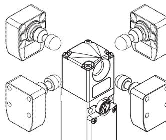
The head can be quickly positioned on all four sides by turning the 4 fixing screws. The lock release devices and the release push-button can also be adjusted by 90° at a time, thus obtaining as many as 16 different configurations with the same article.
