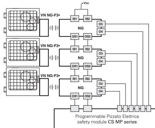
Possible connection in series of several switches in order to simplify the safety system wiring, prior evaluation of the outputs of the last switch in the chain by means of a Pizzato Elettrica CS MP safety module, which allows management of the safety function as well as the signalling function.
