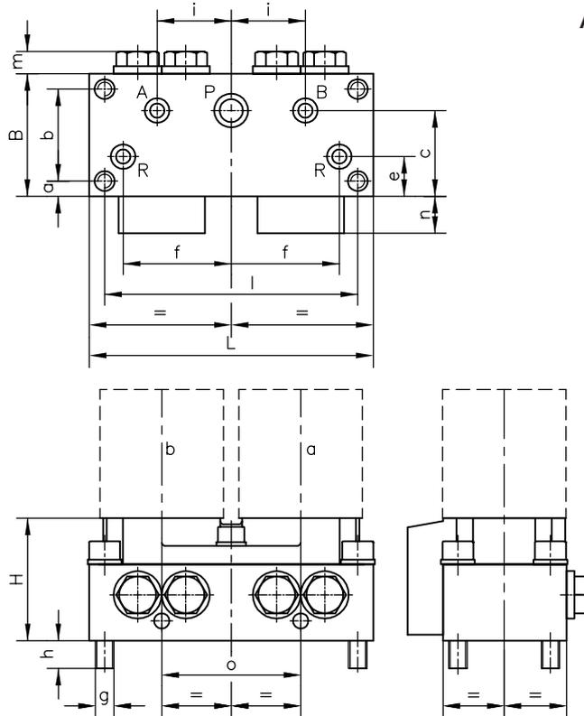
**Attention:** Both return ports R have to be connected, as there is no internal connection.
