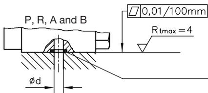
Holes in the manifold and sealing of the ports by O-rings <sup>1)</sup>
