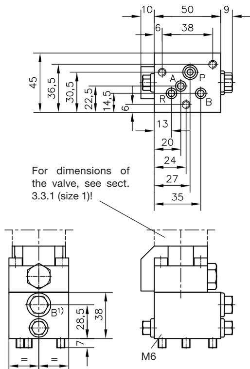
Holes in the manifold and sealing of the ports by O-rings 2)
