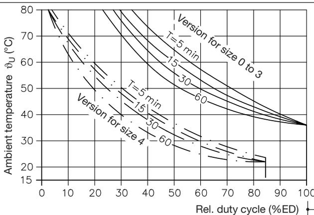
The curves do apply to stand-alone, individual valves only! If the valves are installed in a cabinet, it should be always equipped with louvers! In case of bank arrangement and ambient temperatures above 40°C the layout should be designed in such a way that adjoining solenoids are not energized over prolonged periods.
