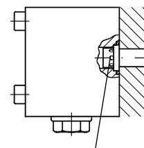
Check valve insert type ER 21 (not available with coding Y, see also sect 2.1, table 2).
