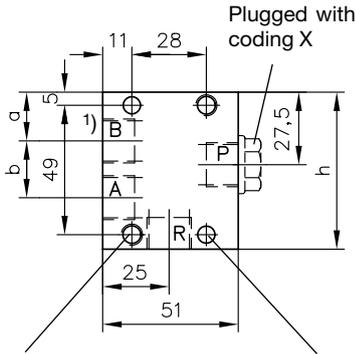
M 8, 10 deep, core bore  $\varnothing 6.5$  is a thru-hole
