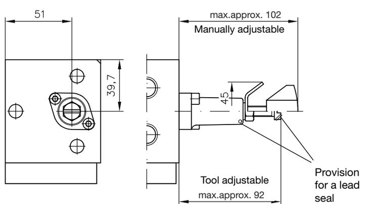
Pay attention to the differing dimensions of the base plate for the pressure compensated version with pressure actuation (see D 6250).
