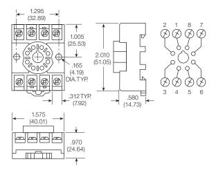
Screw terminal, DIN rail, snap-mount socket 27E892 Offers screw termination for KRPA relays and other devices with 11-pin undecal base. This socket is constructed with a spring-loaded latch which allows it to be quickly snapped onto or removed from a DIN or "top hat" style mounting track. No special tools or extra hardware is required for installation. Sockets have M3.5 screw terminals which accept up to two #12 AWG wires.
