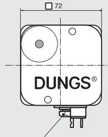
Plug connection for socket according to DIN EN 175 301-803
