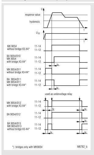
On model BA 9054/6\_\_ with manual reset the contacts remain in the fault state after detecting a fault or after to has elapsed. The contacts are reset by disconnecting the supply voltage.
