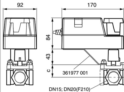
M4R 4-way control valves with actuator ASM 105/115
