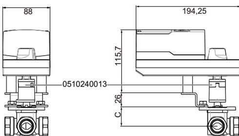
M4R 4-way control valves with actuator ASM 124
