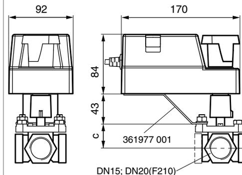
3-way control valves with actuator ASM 105/115
