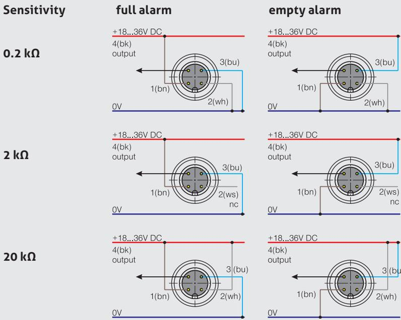
Configuration of the MNV level transmitter with NVS-181/M; NVS-183/M; NVS-186/M
